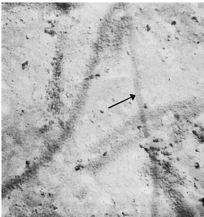
Fig. 7. Electron micrograph of collagen fibrils from hide powder grafted with 20% PMMA (sample G 1 C 1 ) shadowed with palladium-gold. 22,500 \times
